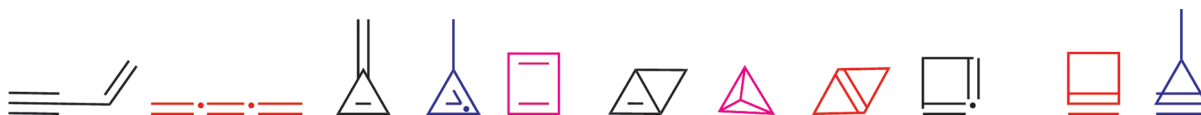
Scheme 1. Lewis Structures of the 11 Possible C 4 H 4 Isomers with Filled Valence Shells a
